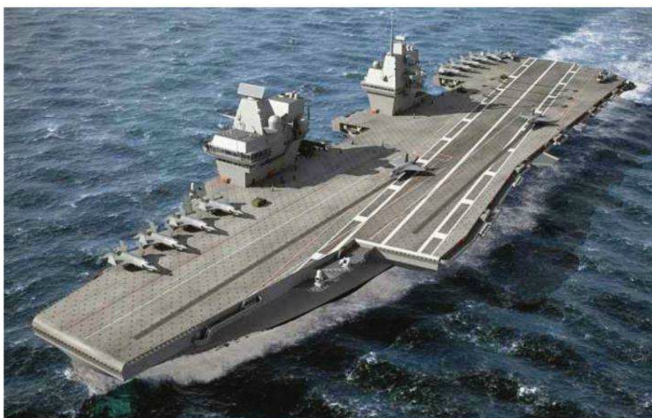
An artist's impression of the Queen Elizabeth-class aircraft carrier design for the RN as amended post-SDSR 2010 to incorporate catapults and arrestor wires for the F-35C carrier variant of the Joint Strike Fighter.
