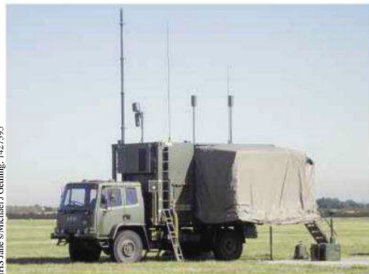
An RAF Regiment Leyland DAF 4x4 truck of the RAF Regiment, mounting a 14ft container housing an Integrated Biological Detection System. The RAF Regiment will soon be the UK's sole active-duty CBRN reconnaissance unit.
