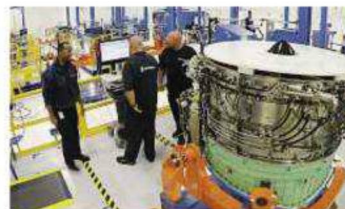
Rolls-Royce employees work on the first fully assembled production-model F-35B lift fan at the company's factory in Plainfield, Indiana.
